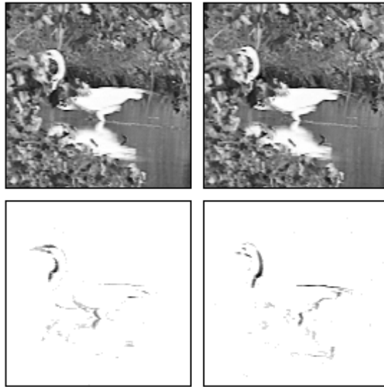
Figure 1: Natural time varying images are highly correlated in space and time. Shown on the top, are two frames of a motion scene separated by thirty three milliseconds. These two frames are highly repetitive, in fact the light intensities of most corresponding pixels are similar. Shown on the bottom, are light increase (on the left) and light decrease (on the right) of the above two snapshots indicated by greyscale of pixels (white means no change). One can immediately see that only a small portion of the image changes significantly over this time scale.
